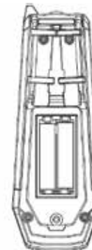
With Battery Cover Removed showing batteries inside
